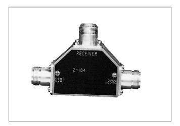
The Z-164A is used as a matching pad for applying the mixed output of two signal generators to the input terminal of a receiver for measuring two-signal characteristics (such as the blocking and intermodulation characteristic) of the receiver.
