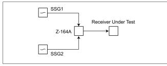
**Connection for Measuring Two-signal Characteristics**
