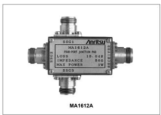
The MP659A and MA1612A are used as an impedance matching box applying the mixed output of three RF signal generators to a receiver input terminal for measurement of three-signal characteristics (such as receiver SINAD performance).
